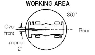
Without outriggers "Over front" operation should be performed within 2 degrees in front of chassis.
